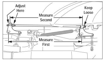
Figure 37. Measure & Adjust Lift Rod Timing
